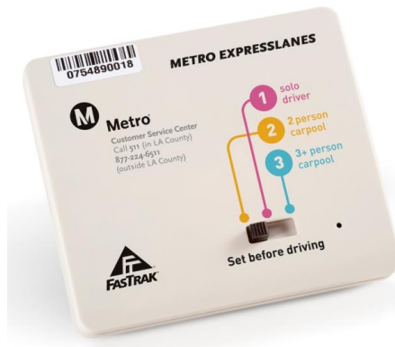
Figure 2-4 Transponder with Occupancy Switch
