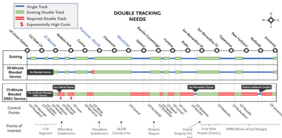
Figure 3: Double-Tracking Needs for Constrained Scenario with 60-Minute Reverse Headways
