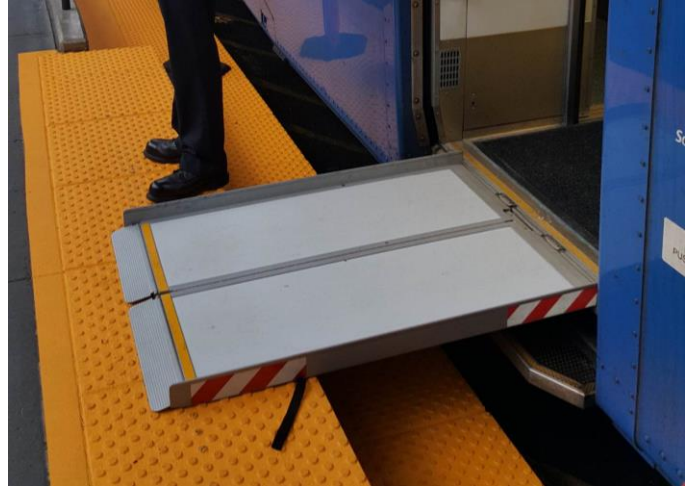
Figure 5 - Manual Boarding ramp used on the Seattle Sounder commuter service
