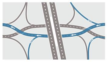
The road geometry, signs, and pavement markings all work together to make circulation very simple. Drivers have responded well to DDIs in cities that have utilized them.
