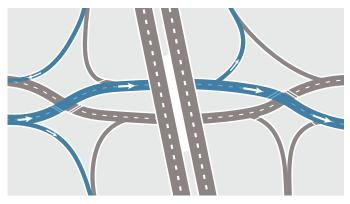
When exiting the interstate onto the local road, motorists are able to make right turns and left turns easily. DDIs reduce the number of points where vehicles cross paths from 10 down to two. This makes the intersections safer for motorists and pedestrians who will have their own signal as well. See diagram below.
