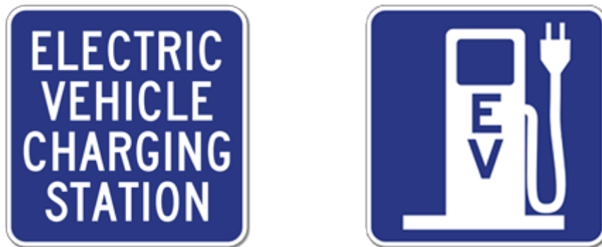
Figure 4. FHWA-approved descriptive wayfinding sign (D9-11bp, left) and symbolized EV wayfinding sign (D9-11b, right).
