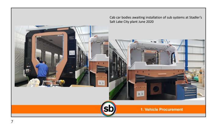
The cars are articulated (share trucks) and thus are semi-permanently coupled. This picture shows the articulation joint on a cab car. The other half of the joint is on the power pack.
