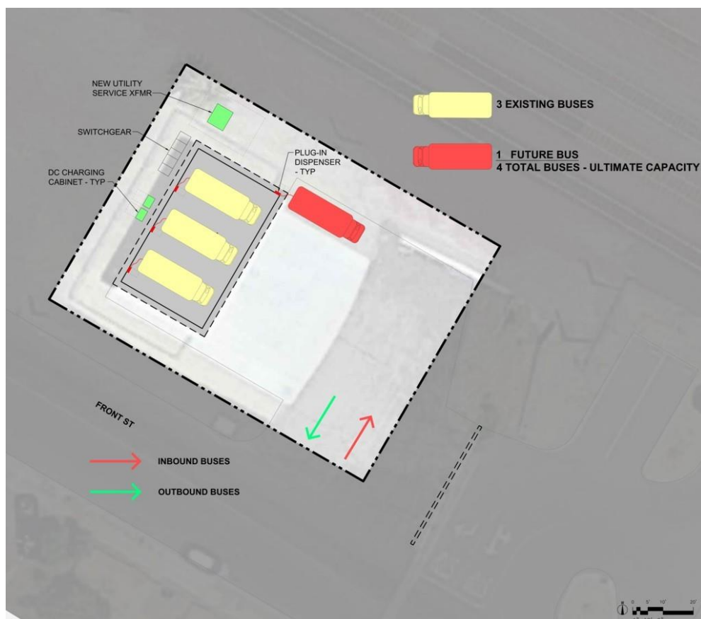
Figure 6-5. NAT Garage - Full ZEB Build-Out
