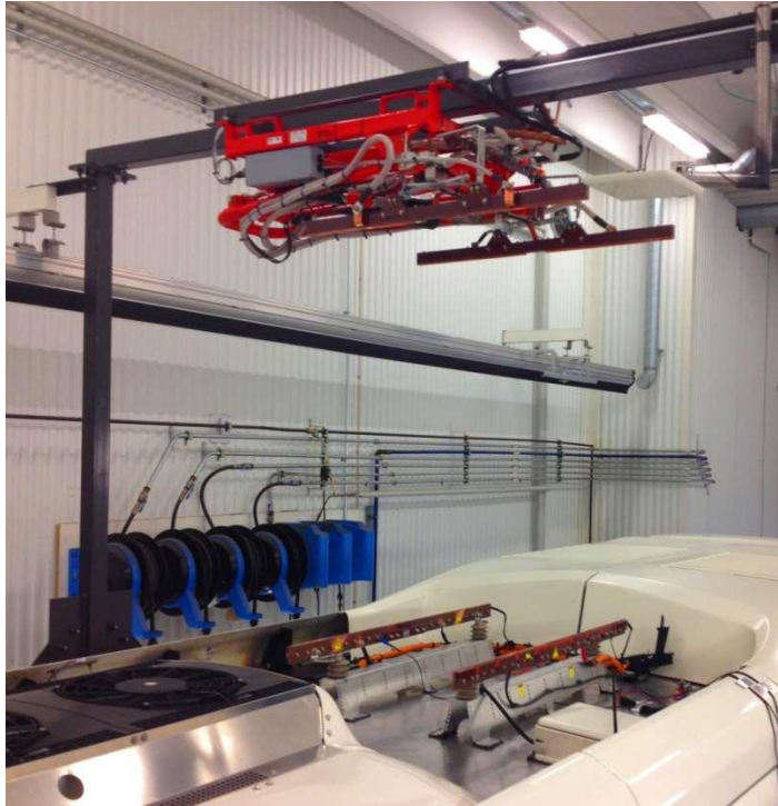
Figure 5-3. Inverted Pantograph and Charge Rails
