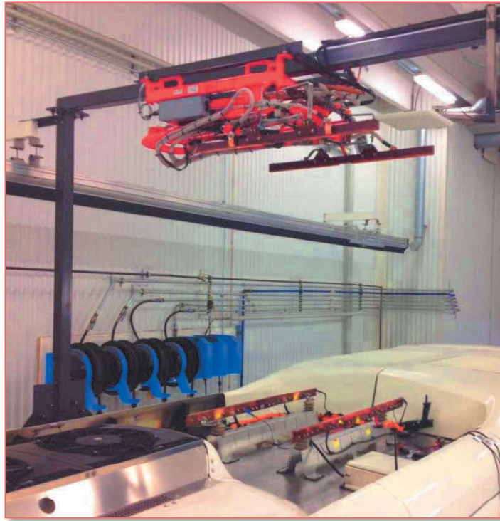
Figure 4-2. Inverted Pantograph and Charge Rails
