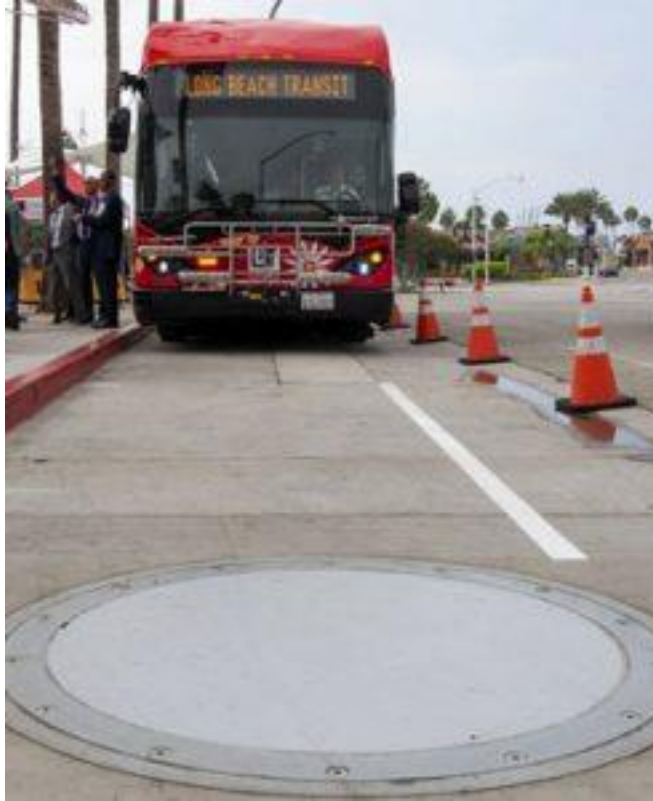
Figure 1-20: Long Beach Transit's WAVE Charger
