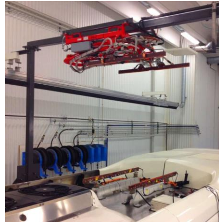
Figure 1-11: Inverted Pantograph & Charging Bars on Bus Roof
