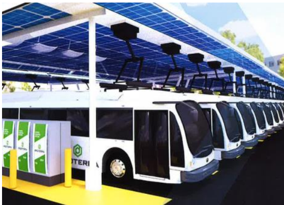
Figure 1-12: Depot Charging with Inverted Pantograph
