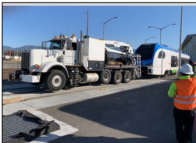
SCRR Brandt truck towing DMU to demonstrate ability to recover the car in case of malfunction
