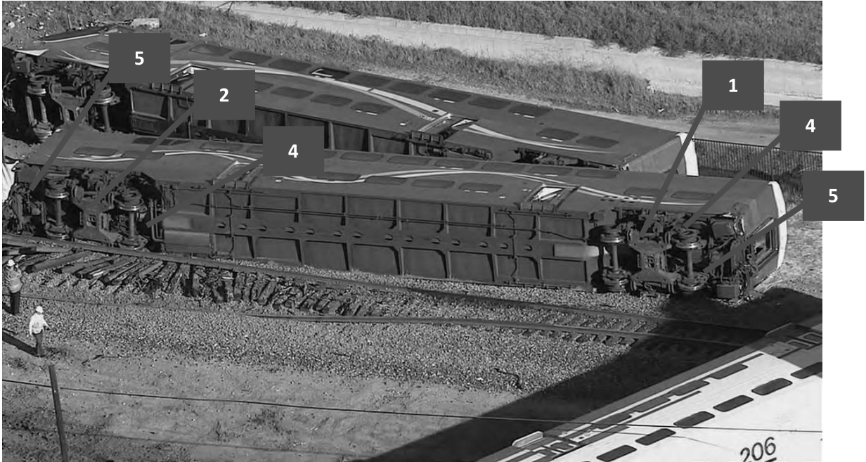
Figure 4.3.5. 3 - #211 ROTEM TRAILER CAR (Underfloor air piping and cabling)
