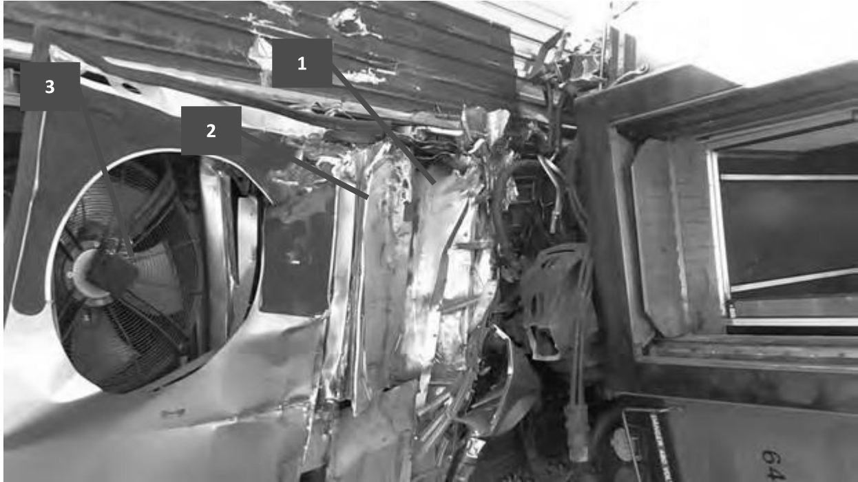
Figure 4.3.4. 2 - #211 ROTEM TRAILER CAR (A-END HVAC Roof Assembly)
